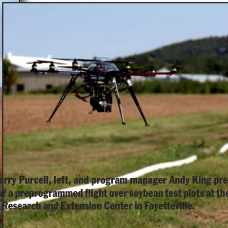
The Oktokopter flies a preprogrammed pattern over soybean test plots at the Arkansas Agricultural Research and Extension Center in Fayetteville.
